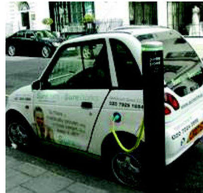
Electric Vehicle Charging Point
